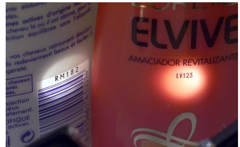
Dating/coding inspection via camera
